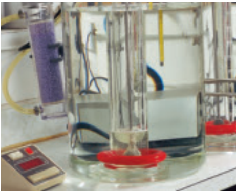
AMSOIL synthetic compressor oils form virtually no foam during ASTM D-892 testing.
